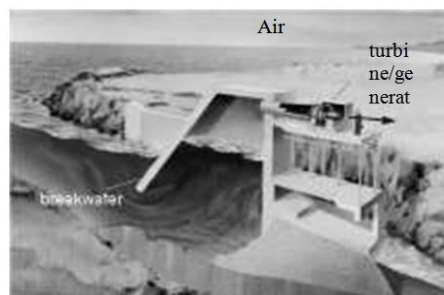
Fig. 5 oscillating column of water system
