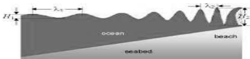
Fig. 3 Formation of a "tsunami"
