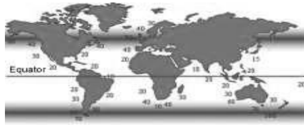
Fig.4 Global wave power distribution in kW/m
